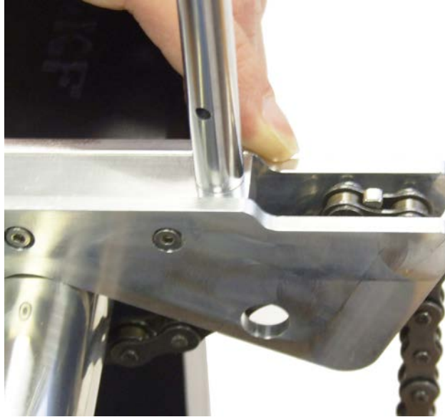
Figure 3 - 9. Attaching the Chain Assembly to the Anchor.
