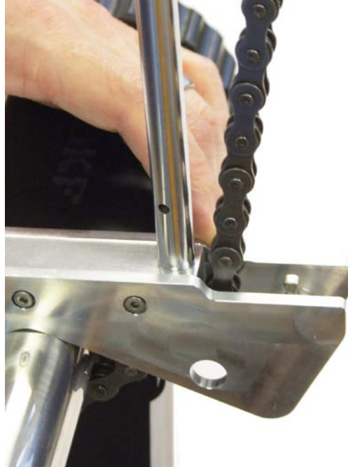
Figure 3 - 11. Tightening the Chain on the Anchor.
