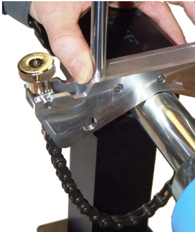
Figure 3 - 10. Attaching the Pivot to the V-Bracket.
