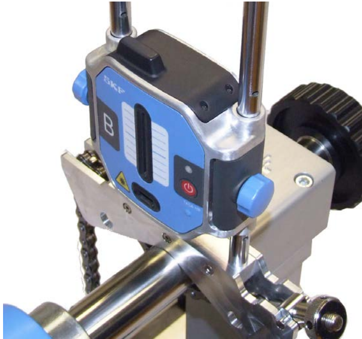
Figure 3 - 14. Measuring Unit Mounted on V-Bracket.
